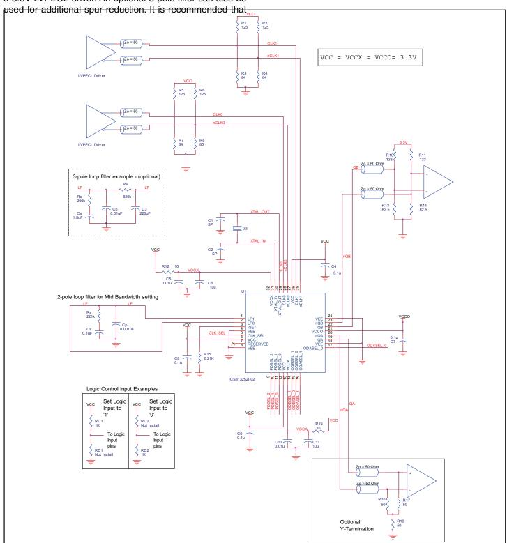
FIGURE 6. ICS813252I-02 SCHEMATIC EXAMPLE
