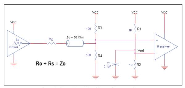
FIGURE 2. SINGLE ENDED SIGNAL DRIVING DIFFERENTIAL INPUT
