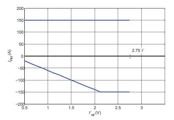
Figure 32: Measuring range versus external  $V_{\rm ref}$  LESR 25-NP
