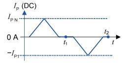
Figure 26: Current cycle used to measure magnetic and electrical offset (transducer supplied)
