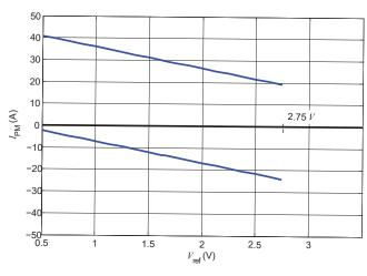
Figure 30: Measuring range versus external  $V_{\mathrm{ref}}$  LESR 6-NP
