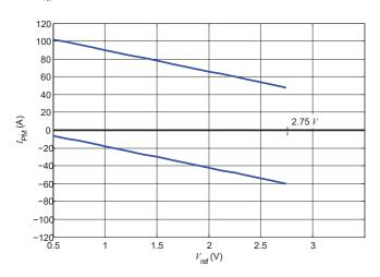
Figure 31: Measuring range versus external  $V_{ref}$  LESR 15-NP
