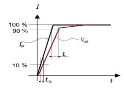
Figure 28: Response time  $t_{\rm r}$  and reaction time  $t_{\rm ra}$
