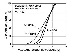
Figure 7. Transfer Characteristics
