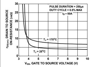
Figure 11. R<sub>DSON</sub> vs. Gate Voltage
