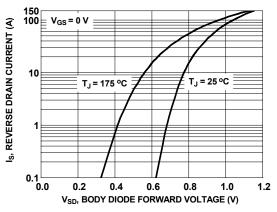
Figure 8. Forward Diode Characteristics
