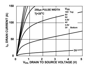
Figure 9. Saturation Characteristics
