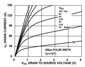
Figure 10. Saturation Characteristics
