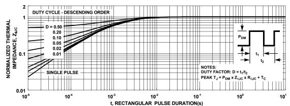
Figure 3. Normalized Maximum Transient Thermal Impedance
