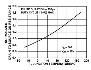
Figure 12. Normalized R<sub>DSON</sub> vs. Junction Temperature
