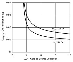
**On-Resistance vs. Gate-to-Source Voltage**
