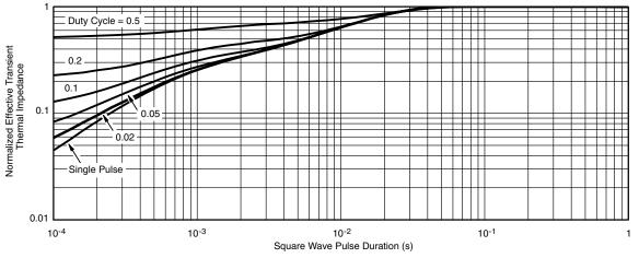
Normalized Thermal Transient Impedance, Junction-to-Case
