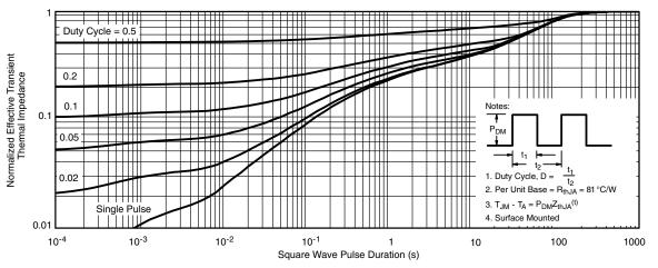
Normalized Thermal Transient Impedance, Junction-to-Ambient
